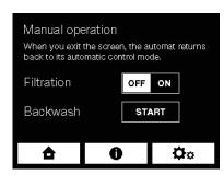
Manual control allows to: **switch filtration on/off** independently to preset filtration periods. **start filter washing** independently to
