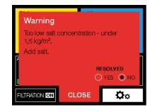
Too low salt concentration in the water. Less than 1.5 kg/m3.
