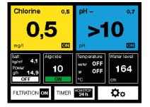
The probe shows a pH> 10 Check the pool water and probe.
