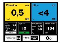
The probe shows pH <4 Check the pool water and probe.
