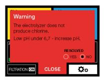
Electrolysis does not produce chlorine. The pH value is below 6.7, increase the pH value.
