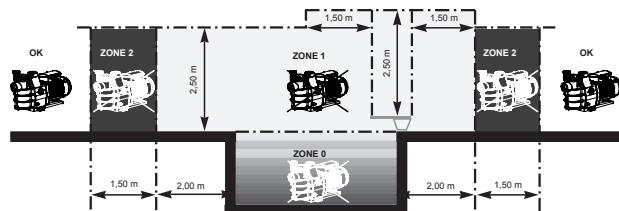
Install the pump in a ventilated and dry place. The motor requires air to flow freely around it to provide for natural ventilation. The pump has to be installed, so that the plug and the wall socket outlet is easily visible and accessible.
